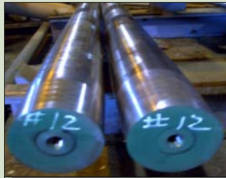
Accurloy piston rods with tapered ends.
